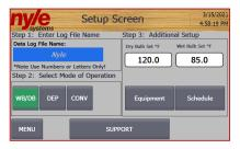
From the Setup screen, the user can set the Log File Name, Select the Mode of operation and navigate to the Schedule and Support Screens.
