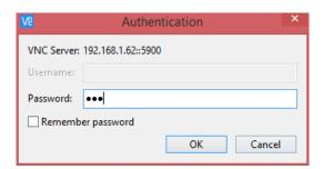
Type in 100 or the defined password and then press OK or enter. This will bring up the same screen that is displayed on the HMI screen and the user will be able to monitor or change values as the user would be able to on the HMI screen.
