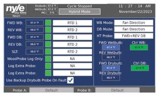
The FWD and REV Dry Bulb and Wet Bulb readings are coming from. The user can also change which probe is the "active" probe based on fan direction. These are all under specific defaults, & changing them will fundamentally change how the kiln operates. For example, changing the WB and DB mode to "OPP Fan Direction" will make the active DB and WB read the air on the exiting side of the lumber stack instead of the entering side.
