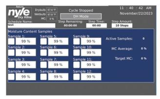
The moisture samples screen allows the user to manually input the moisture content of various samples in the kiln charge. These will directly correlate to MC% steps set up in the schedule. (See schedule section, Page) If the box next to a particular sample is checked, then that sample will be used as part of the average samples calculation. This is the value used for MC% steps in the schedule.
