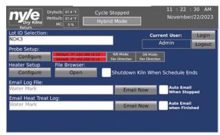
The advanced settings screen allows the user to log in as an operator or admin. It also allows the user to enter a lot number manually, configure which probes the kiln is running off, and set up emails for log files.
