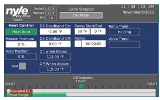
In the heat control screen, specific settings and adjustments for manual operation can be made. Clicking on the heat control box (highlighted green) will open a scroll wheel for heat Auto, Manual, or Off.
