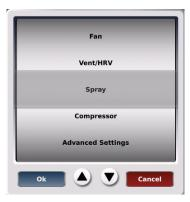
The configure button opens up a scroll wheel list of equipment in the kiln. This allows the user to access much finer degrees of control with these various pieces of equipment. While running the kiln
